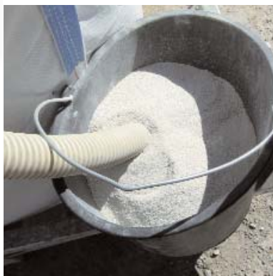
Many subsamples now form a representative sample of the content of the entire bag and are poured into a bucket.
