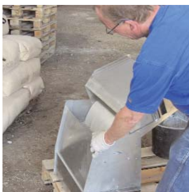
The content of the bucket is split with a device for splitting samples.
