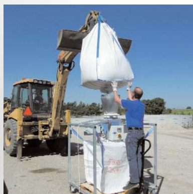
The big bag is emptied through the sampler and into a clean big bag.
