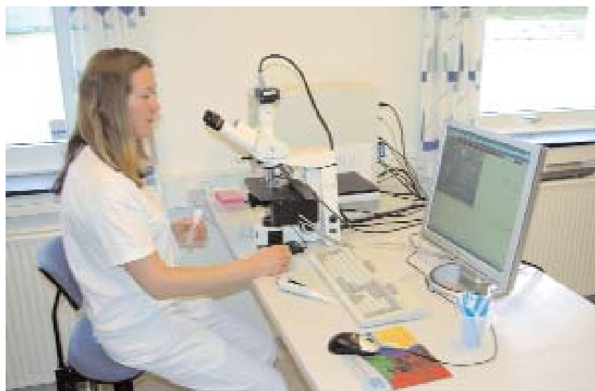
Cicilie at Hatting AI analyses sperm motility with CASA – Computer Assisted Sperm Analysis.
